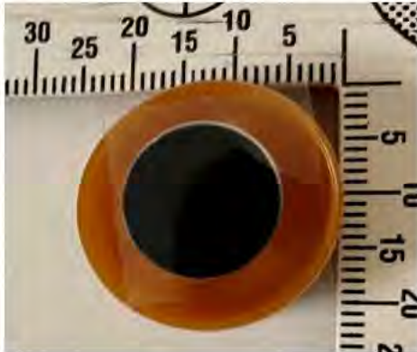
Figure 1: Example SEM stub prior to sample recovery, showing adhesive tape in situ
